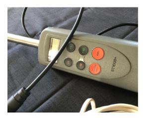
Autopilot for tiller steered sailboats. Max. Displacement 6,600 lbs. Cockpit autopilot Lead-screw and nut drive SeaTalk/NMEA GPS compatible 12 volt DC Backlit LCD display, 6 button Digital Keypad Includes everything needed for installation on your boat. A hard to find autopilot for use on tiller steered vessels. Very low usage hours, excellent condition
