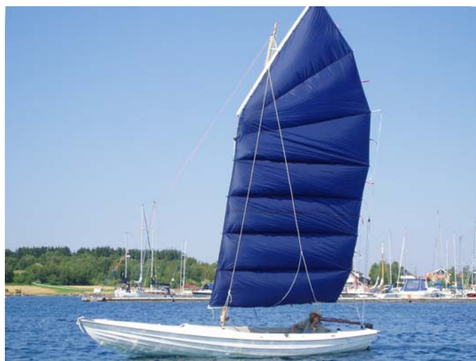
..18ft dinghy Broremann with 10sqm sail. Note the mast lift and simple lazy jacks...
