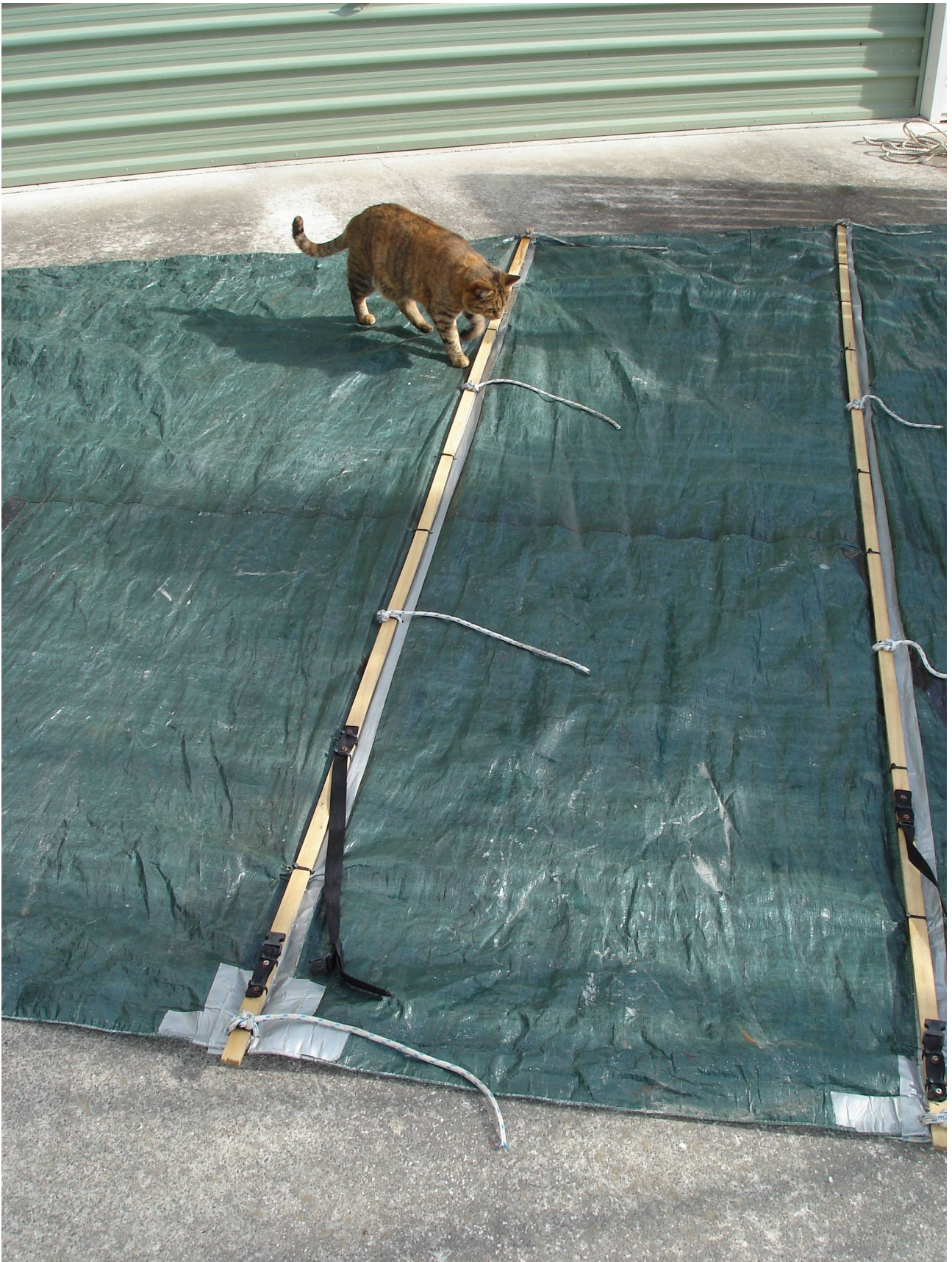
<<Battens.jpg Battens secured using electrical ties. Note fixed parrels and reefing ties.>>
