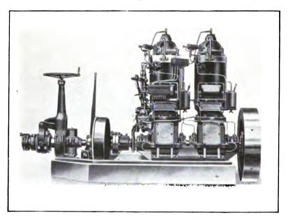
FIG. 7.—Avance 60 B.H.P. Oil Engine, with reversible propeller blades.
