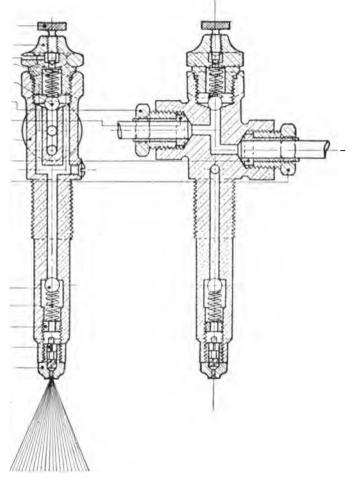
FIG. 119.—Injection Nozzle Avance Engine.
