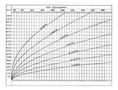
FIG. 169.-Speed and Power Curves for Passenger Vessels.
