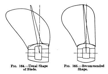
Set-Back.—Propellers for ordinary commercial craft require no set-back at all. Set-back is a disadvantage for going astern and manœuvring, but is probably of value on fairly fast vessels, and any disadvantage in going astern is not important on such boats.
