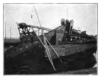
FIG. 305.—Tin Dredger, three 45 H.P. Kromhout Engines.
