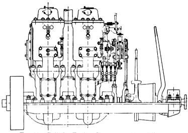
FIG. 13.—Bolinder Engine, direct reversible "E" type.
