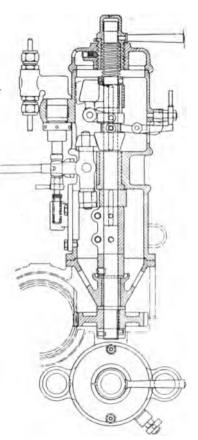
FIG. 127.—Skandia Centrifugal Governor, with Skew Gear.
