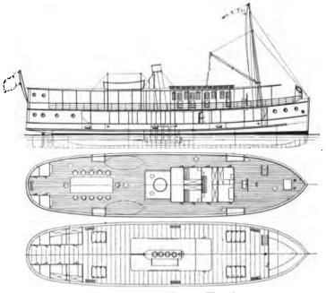
FIG. 264.-Motor Cargo Vessel,
