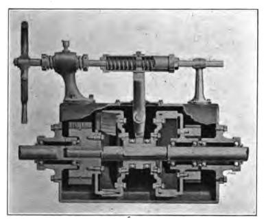
FIG. 95.—Shiners' Patent Reverse Gear.
