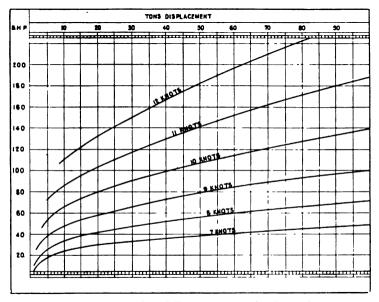
FIG. 173.-Speed and Power Curves for Launches.
