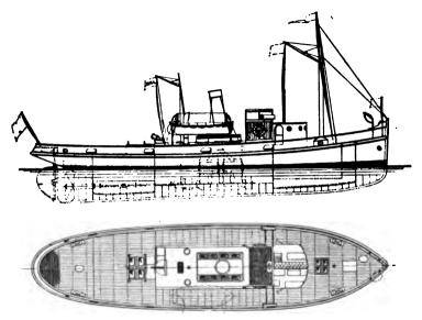
FIG. 220.—Design of Sea-going Motor Tug.
