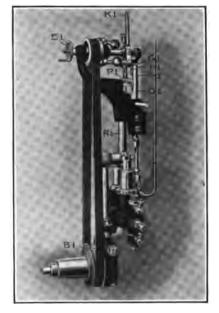
FIG. 118.—Fuel Pump and Governor, Skandia Engine.
