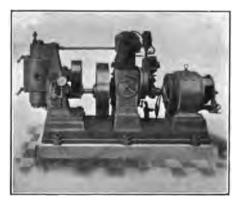
FIG. 365 – Compressor and Electric Generator, driven by Paraffin Engine,
