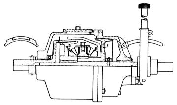
FIG. 87.—Caledonia Reverse Gear.
