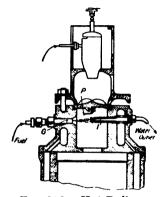
FIG. 106.—Hot Bulb or Plate of the "Original" Hein Motor.
