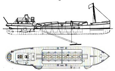
FIG. 307.—Motor Suction Dredger.
