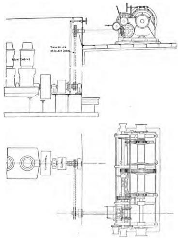
FIG. 249.-Trawl Winch, Chain Drive.
