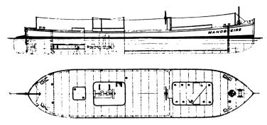
FIG. 259.--Plan of Single Screw Light Draft Motor Barge.
