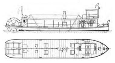
FIG. 268.-Motor-driven Stern Wheeler.
