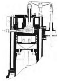
FIG. 67.-Sectional view, Thermomotor.
