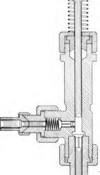
as much as from  $4\frac{1}{2}$  mm. to 2 mm.—the diameters being proportioned to inject the requisite amount of fuel in each case.
