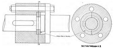
FIG. 147.-Loose Coupling.
