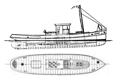
FIG. 221.—Design of River Motor Tug.
