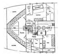
FIG. 236.-Aft Accommodation of Three-masted Schooner.
