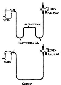
FIG. 348.-Lead of Fuel Pipe.
