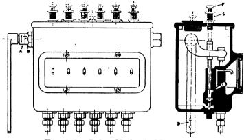
FIG. 152-Robey Mechanical Lubricator.
