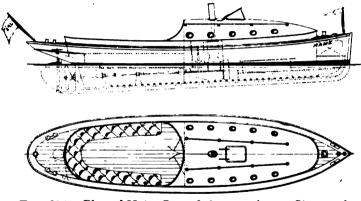
FIG. 284.—Plan of Motor Launch for carrying on Steamers' Decks.
