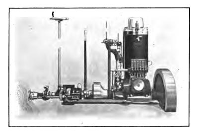
FIG. 64.—Skindia, with reversible blade propeller and centrifugal governor.
