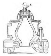
A bulb fitted to the Koch engine, built at Zurich, in Switzerland, is illustrated in Fig. 102, from which it will be seen that the hot bulb (e) is practically surrounded by water, and that there is a  $\cdot$ sort of sluice valve (b) which is operated by hand, so as to control the level of the water. In this way the temperature of the hot bulb is regulated according to circumstances. The fuel
