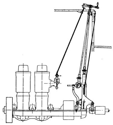
FIG. 148-Deck Control Gear.
