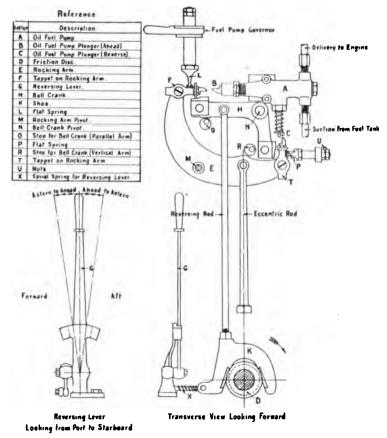
FIG. 81.—Diagrammatic Sketch, Bolinder Direct Reverse.
