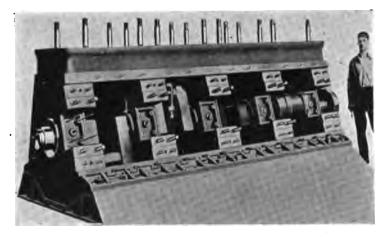
FIG. 72.-Weiss Accessible Crankshaft.
