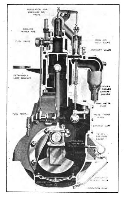
FIG. 21.-10 H.P. Cross Engine, end view.
