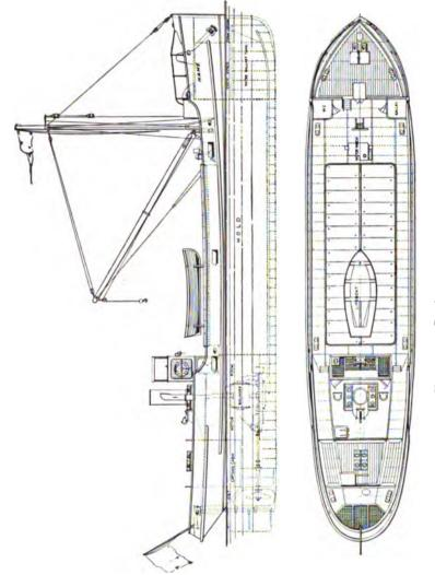
FIG. 194.-Design of Motor Coaster.
