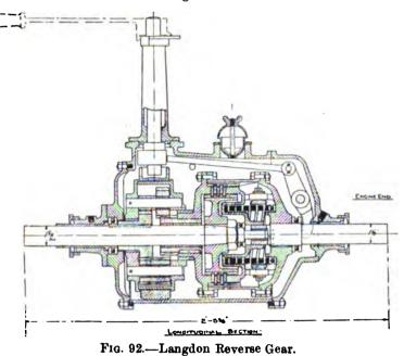
Langdon Gear.—Fig. 91 is a sectional elevation of this firm's old type of gear. Locked ahead drive is produced when
