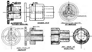
FIG. 145.-Langdon Patent Sleeve Coupling.
