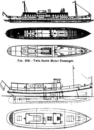
FIG. 310.—Passenger Boat, Dan Engine.
