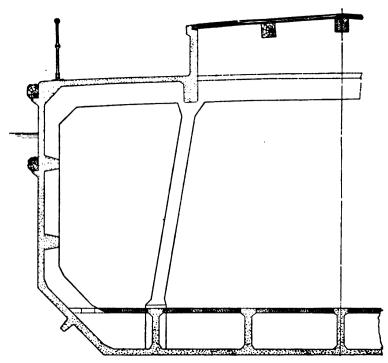
FIG. 2)2.-Section of Pollock's Reinforced Concrete Coaster.
