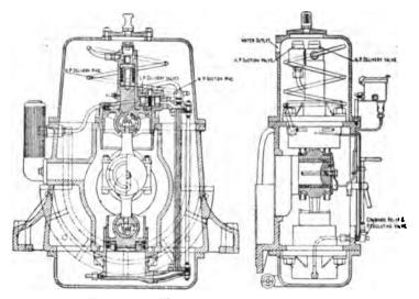
FIG. 367.-Three-stage Air Compressor,
