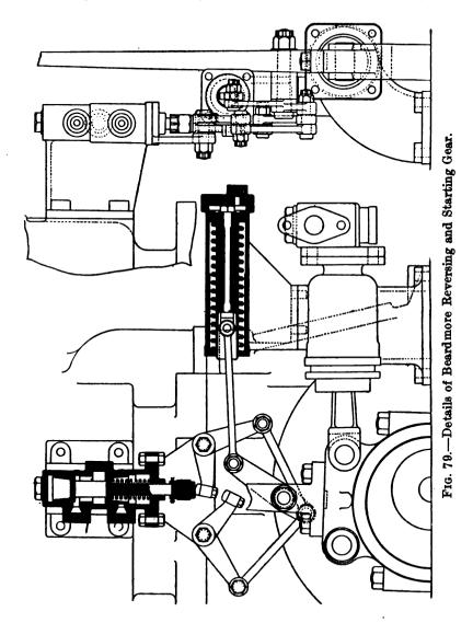
piston in a horizontal cylinder. This horizontal cylinder can be put in connection with the atmosphere or with the  $H^2$
