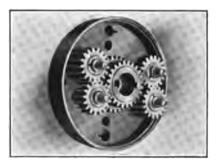
wheels and the FIG. 86.—Pinions of Ideal Reverse Gear. detail design, but more
