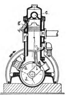
FIG. 70.—Section of Tuxham Engine
