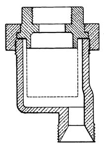
FIG. 331.—Pipe Filter.
