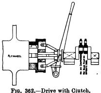
FIG. 302.—Drive with Clutch,
