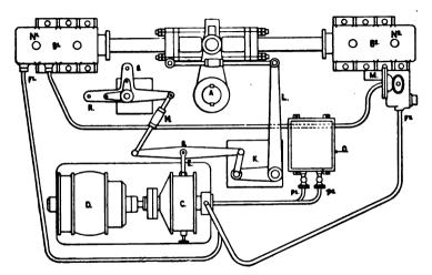
FIG. 355,-Hele-Shaw Electric Hydraulic Steering Gear.
