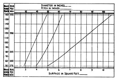
FIG. 163.—Propeller Curve, Single Screw Coasters.
