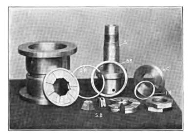
FIG. 136.-Michell Thrust Bearing.
