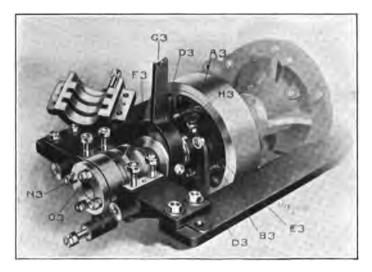
FIG. 134 .- Skandia Solid Thrust Block and Clutch.
