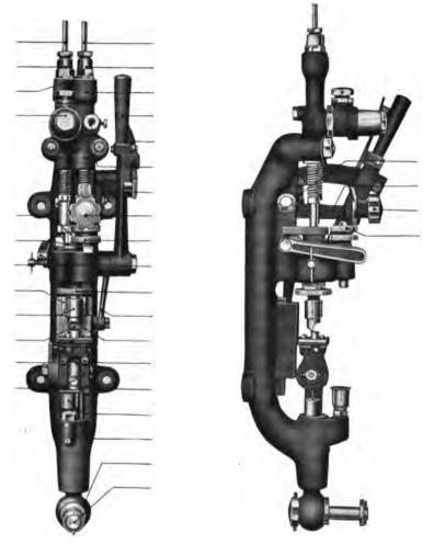
FIG. 114.-Fuel Pump, Avance Engine.
