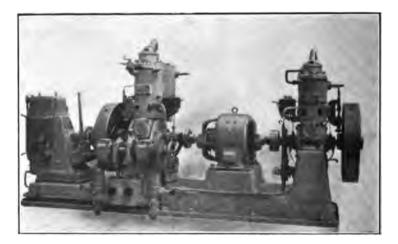
FIG. 358,--Combined Air Compressor and Electric Generating Set, with Kromhout Engines.
