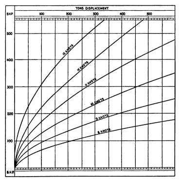
FIG. 172.-Speed and Power Curves for Yachts.
