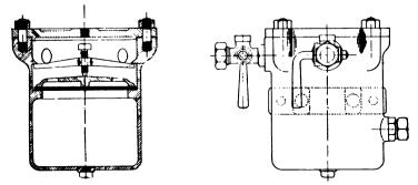
FIG. 329.-Gauze and Cloth Independent Filter.
