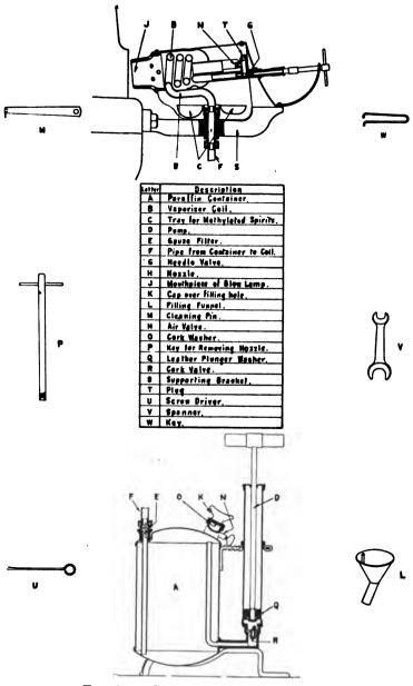
FIG. 156.—Pressure Lamp and Container.
