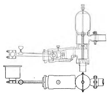
FIG. 369.-Bilge Pump driven off Pin on Flywheel Cap.
