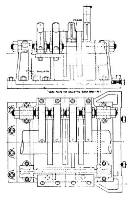
FIG. 135.-Adjustable Thrust Block.
