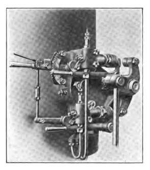
FIG. 116.—Petter Fuel Pump Gear.
