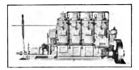
FIG. 46.-Mietz and Weiss Oil Engine, with reversing gear.
