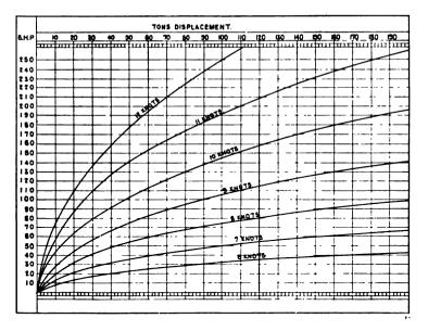
FIG. 174.-Speed and Power Curves for Fishing Vessels.
