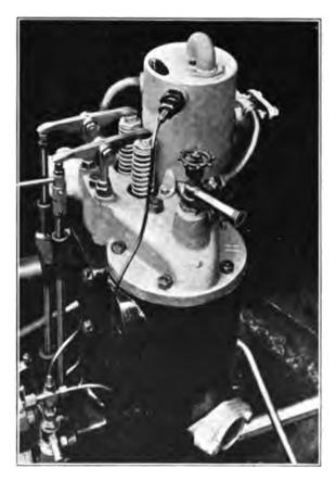
FIG 34.- Hein Oil Engine, valves and cylinder head.
