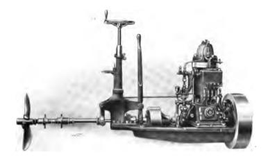
FIG. 28.—Dux Oil Engine, with reversible blades.
