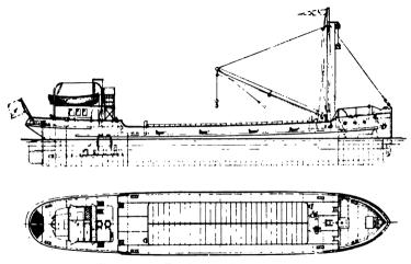
FIG. 195.—Design for Motor Coaster.
