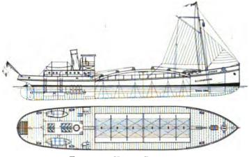
FIG. 308.—Hopper Barge.
