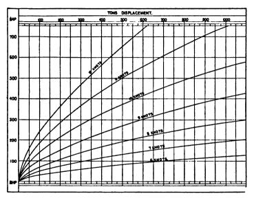
FIG. 170.—Speed and Power Curves for Motor Coasters.
