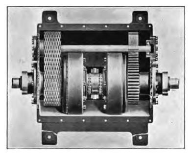
FIG. 94.-Shiners' Patent Reverse Gear.
