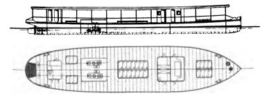
FIG. 260.—Plan of Twin Screw Light Draft Motor Barge.
