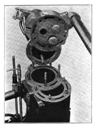
FIG. 35.—Hein Oil Engine, with cylinder head removed.
