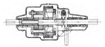
FIG. 89.-Gaines "B" Type Reverse Gear.
