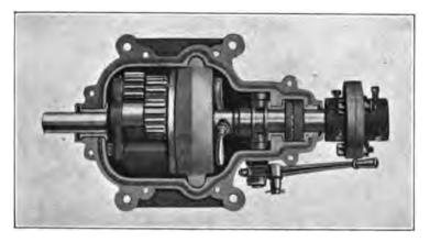
FIG. 88.-Gaines "B" Type Reverse Gear.
