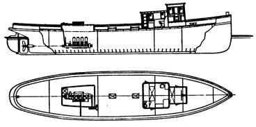
FIG. 313.-General Arrangement of Water Boat Aquadon.
