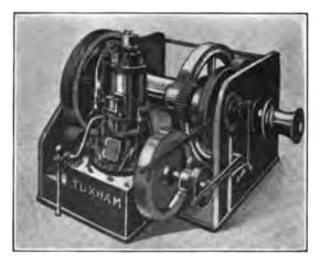
FIG. 349.--Tuxham Oil Engine Winch.
