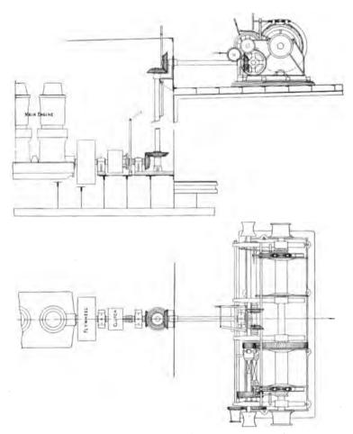
FIG. 248.-Trawl Winch Drive from Main Engine.
