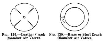
Many makers at one time fitted leather flap valves (see Fig. 129). These worked satisfactorily whilst they remained
