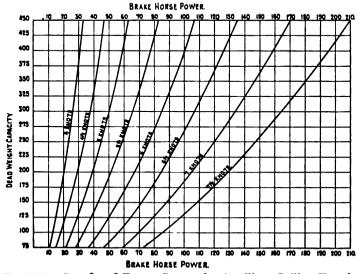
FIG. 176.-Speed and Power Curves for Auxiliary Sailing Vessels.
